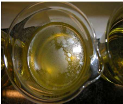
Two examples of B5 samples with a floating layer at the top.
