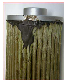
Picture: contamination found in oil filter!
