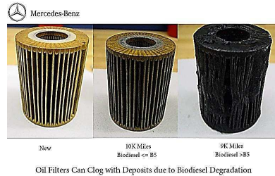
Picture: oil filter clogged after 9k miles using > B5 diesel.
