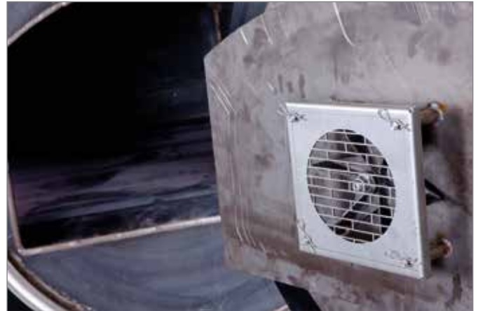
Circulation fan in the furnace door
