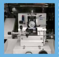
use of the attributes of a FeatherTM blade, the Quick Release FeatherTM blade Holder enables the cryotomist to use the full length of the blade without waste. Other important features are the fact that the blade angle can be changed without changing the position of the blade
