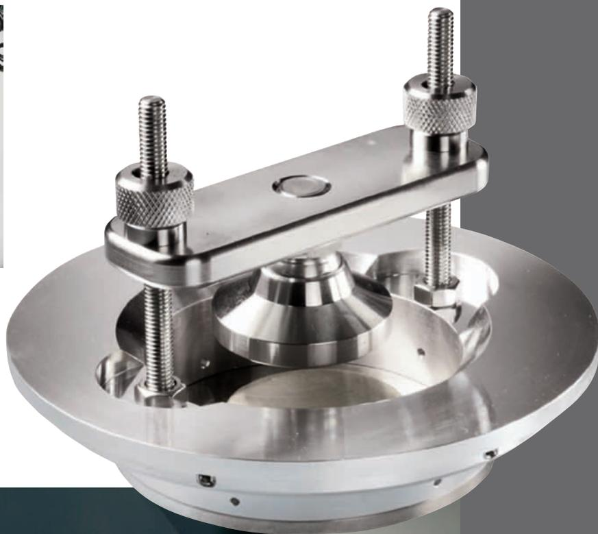
Figure 2: Placement of the sample holder in the GD source
