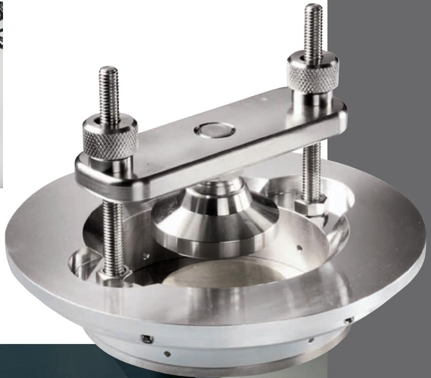
Figure 2: Placement of the sample holder in the GD source
