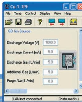
Figure 11: Glow Discharge Ion Source software control
