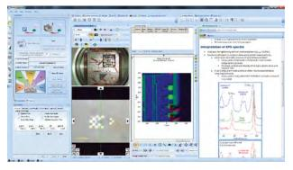
to transfer samples is defined by the monitored pressure in the system, set to ensure that out-gassing samples remain in the load-lock until they are ready to analyze. Avantage monitors all system parameters, storing the data to keep a record of the performance of every system component, and can automatically calibrate Nexsa with a single button press.
