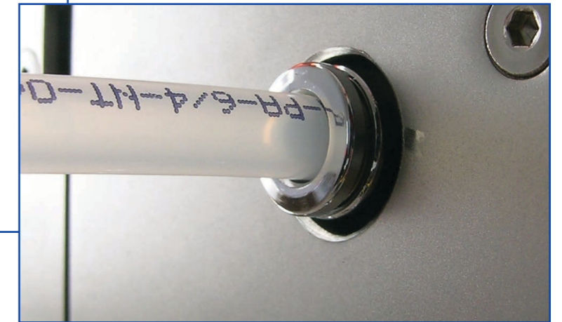
External gas supply at HGC 30
