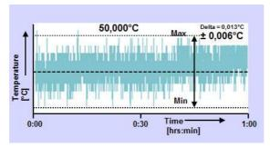
This is the real difference between the minimum and maximum temperature for 60 minutes. Some competitors just state the standard deviation of the mean or mention the stability for a few minutes.
