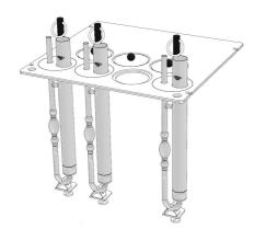
The cover of the bath has round 51 mm holes with lids, for suspending glass capillary viscometers in holders.
