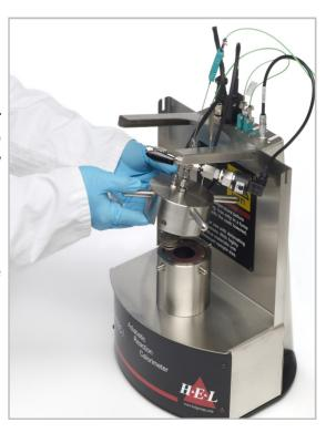
The entry level Phi-TEC I uses high pressure cells, or bombs, of between 7-11ml volume to determine the heat evolved and pressure developed during the reaction. Sample sizes from 0.5 to 5g are typical.
