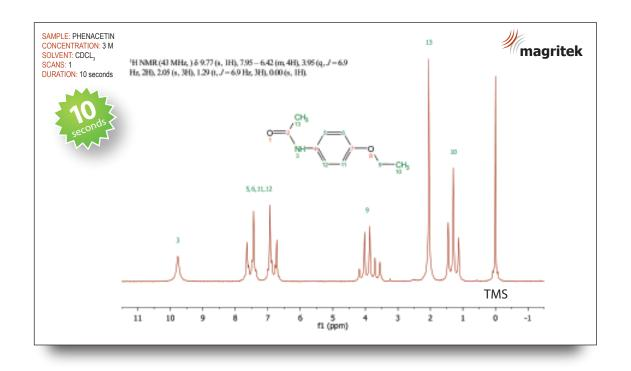
In the second spectrum the student checks if their final product is phenacetin. Note the obvious appearance of the methyl peak at 1.3 ppm and the methylene peak at 3.9 ppm, as well as the disappearance of the hydroxyl peak at 8.4 ppm.
