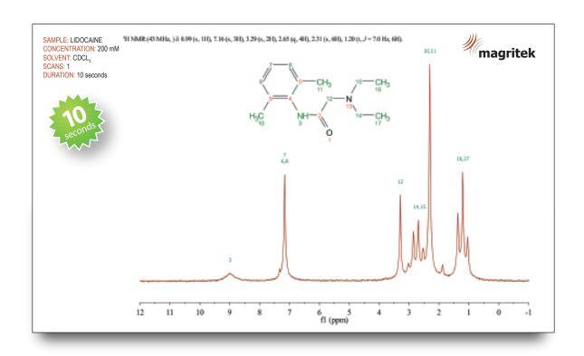
Shown here is an example spectrum of a 200 mM lidocaine sample dissolved in d-chloroform and measured in just 10 seconds. All the spectral features can be observed and resolved. The methyl groups at positions 16 and 17 are resolved completely from the methyl groups at 10 and 11.
